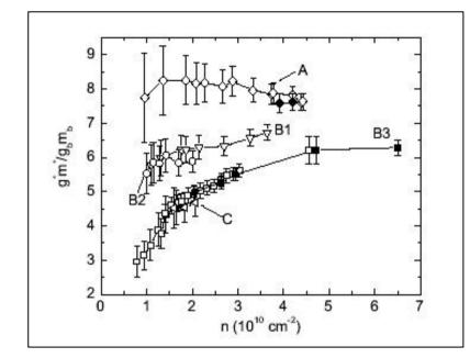
g<sup>\*</sup>m<sup>\*</sup>/gm is strongly sample dependent, signaling that the orbital effects are the origin for the enhanced m<sup>\*</sup>. The effective mass m<sup>\*</sup> = m<sub>b</sub> for electron densities  $2.7 * 10^{10} < n_s < 4.2 * 10^{10} cm^{-2}$ .
