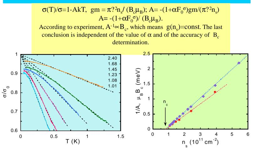
Sharp increase of the effective mass near the critical density in a metallic 2D electron system.
