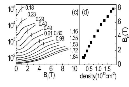
$m^*g^*/m_bg_b$  obtained from SdH oscillations and from resistance saturation.
