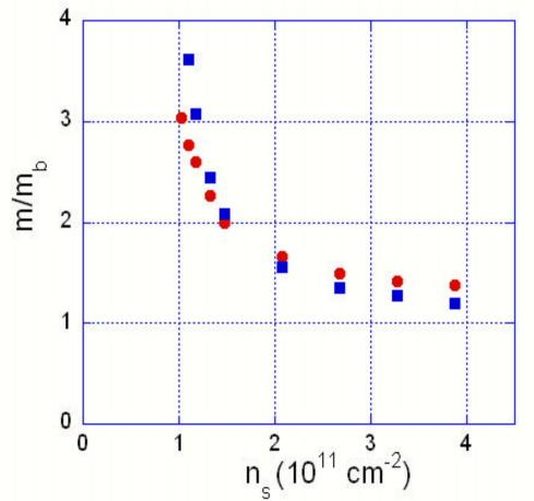
The effective mass determined from the analysis of the parallel field magnetoresistance and temperature dependent conductivity (squares) in comparison to the one extracted from the analysis of SdH oscillations (circles).
