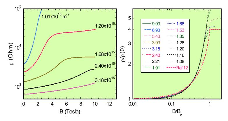
Critical magnetic field as a function of electron density. A.A. Shashkin, S.V. Kravchenko. V.T. Dolgopolov, and T.M. Klapwijk, PRL 87, 086801 (2001).
