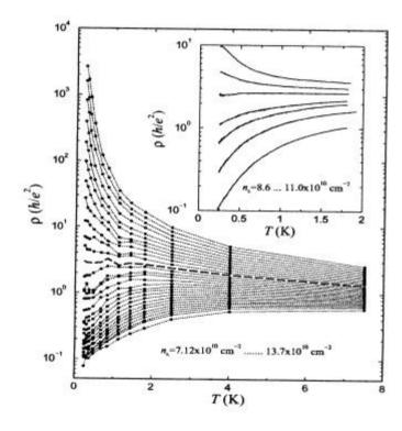
Temperature dependence of the resistivity in a dilute low-disordered Si MOSFET. (from Kravchenko et al., 1995)
