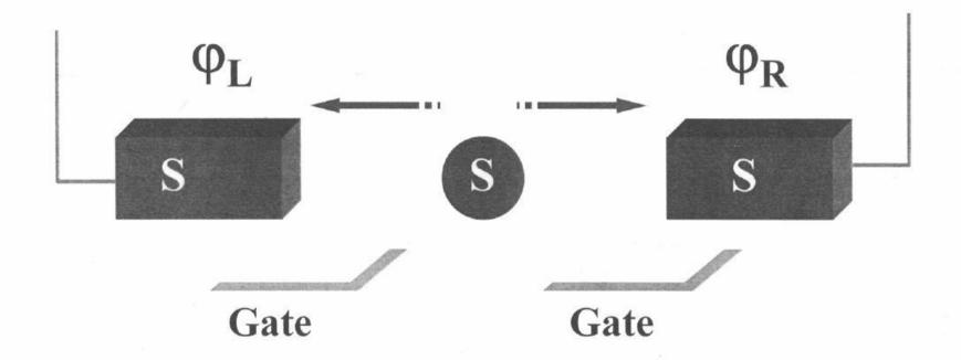
A single Cooper-pair box, by periodically moving between two superconducting leads, is able to keep phase coherence of the two distant electrodes
