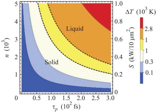
Fig. 2. The temperature change of the NP for its plasmon population during the pulse versus the pulse duration. The area between dashed lines denotes the partial melting region. Right axis shows corresponding power of the driving laser beam. The parameters are as for the Fig. 1, with the standard thermal constants of gold [20]
