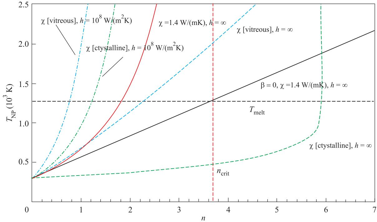
Fig. 1. (Color online) The steady-state temperature of the NP versus the number of plasmons. Parameters used:  $a = 10 \text{ nm}$ ,  $\hbar\omega = 1.9 \text{ eV}$ , and  $T_0 = 300 \text{ K}$ . The gold melting point is taken to be  $T_{\text{melt}} \approx 1270 \text{ K}$  [20]
