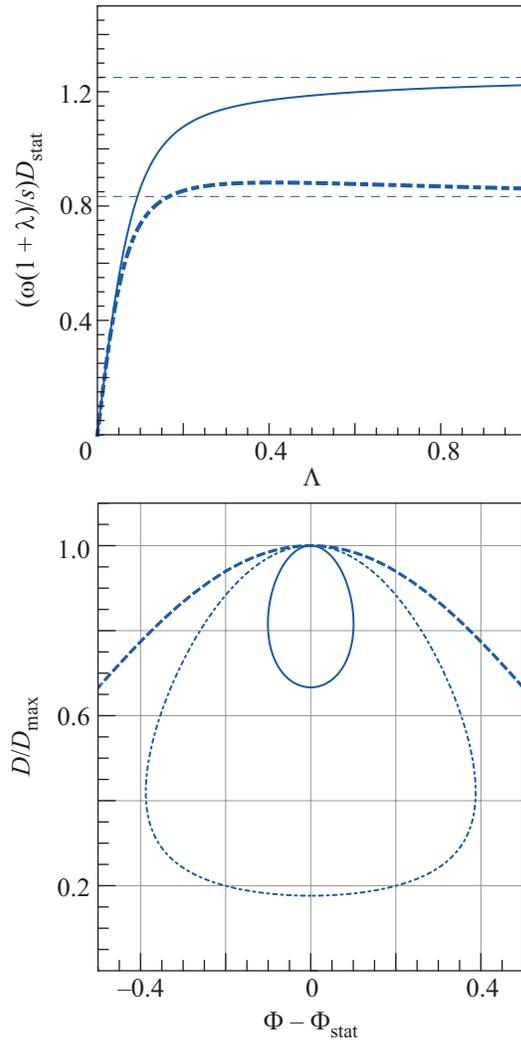
Fig. 1. On the top: dependence of Taylor deformation parameter  $D_{\text{stat}}$  on  $s$  and  $\omega$  at small  $\lambda$  (dotted line) and large  $\lambda \gg 1$  (solid line), plotted in appropriate axes for  $(1 + \lambda)\omega/s \gg 1$ . On the bottom: correlated oscillations of capsule form and inclination angle, where  $\Phi$  is measured in radians, for  $D_0/D_{\text{stat}}$  be equal to 0.2 (solid line), 0.7 (dashed-solid line) and 1.3 (dashed line)
