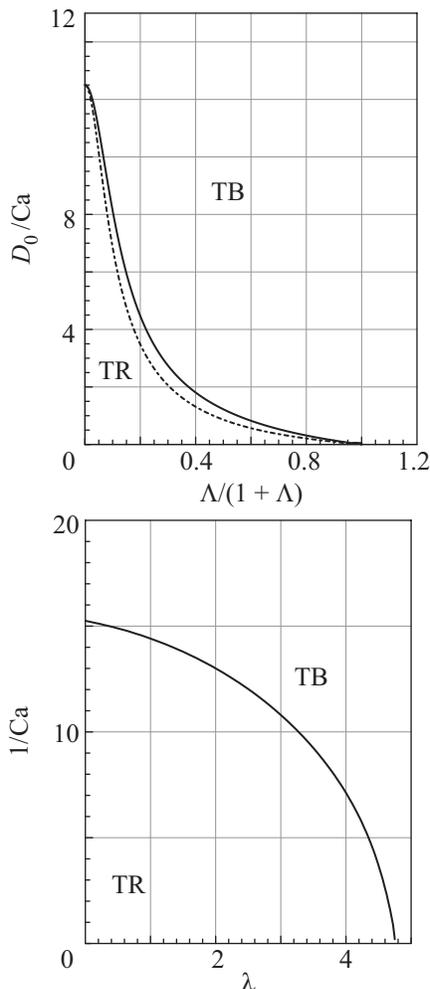
Fig.2. On the top: phase diagram for capsule dynamic regimes plotted in universal dimensionless variables. Solid line is for limit  $\lambda \gg 1$ , dashed – for  $\lambda \ll 1$ . Lines correspond to transition from tumbling, which is under line, to trembling, which is realized above line. On the bottom: phase diagram plotted for shear flow  $s = \omega = \dot{\gamma}$ . Taylor deformation parameter at the rest is  $D_0 = 0.2$
